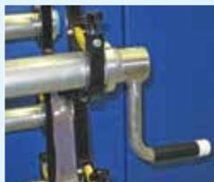
Two hand cranks with rotating grips for easy winding
