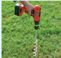
**3.** Mark and drill holes for poles with 18" auger (included).
