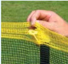
**2.** Attach fence fabric to top cap with easy open/close latch.
